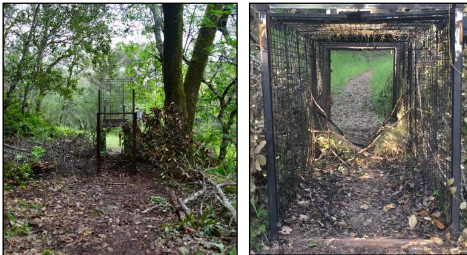
Figure 1. Mountain lion cage trap set on a path (left) with detailed setting using stepping sticks with no treadle-plate (right).
